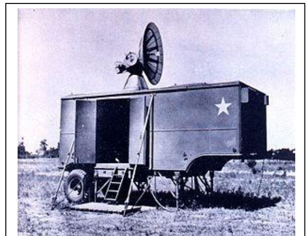
This SCR-584 fire control radar for artillery was deployed in vast quantities
