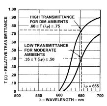
Figure 6. Typical Transmittance Curves for Filters to be used with Standard Red Displays.
