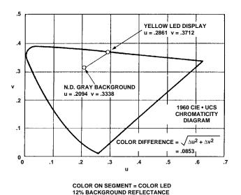
$IDC = \frac{\sqrt{\Delta u^2 + \Delta v^2}}{0.027}$   $\sqrt{\Delta u^2 + \Delta v^2} = 0.0853$   $IDC = \frac{0.0853}{0.027}$  IDC = 3.16
