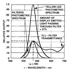
Figure 11. Effect of a Wavelength Filter on a Yellow LED Display.
