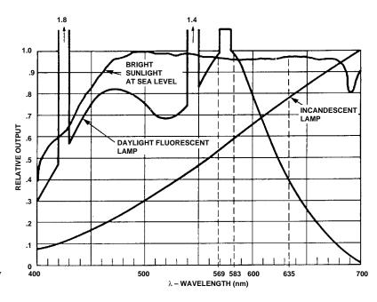
Figure 16. Spectral Distribution for Sunlight, Daylight Fluorescent and Incandescent Ambient Lighting.
