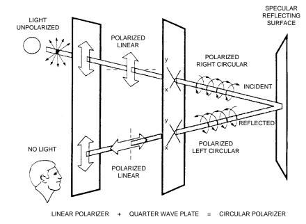
Figure 35. Operation of a Circular Polarizer.
