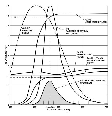
Figre 14. A Neutral Density Gray Filter in Combination with a Light Amber Filter for Use with Yellow Displays.
