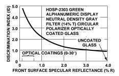
Figure 45. Effect of Reducing Front Surface Reflectance.
