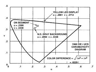
COLOR ON SEGMENT = COLOR LED + COLOR REFLECTIONS 12% BACKGROUND REFLECTANCE .7% DIFFUSE FRONT SURFACE REFLECTANCE
