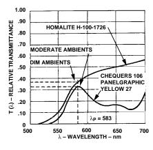
Figure 8. Typical Transmittance Curves for Filters to be used with Yellow Displays.
