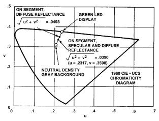
COLOR ON SEGMENT = COLOR LED + COLOR REFLECTANCE BACKGROUND = 25% SPECULAR REFLECTANCE .8% DIFFUSE REFLECTANCE FILTER = .25% SPECULAR REFLECTANCE .02% DIFFUSE REFLECTANCE
