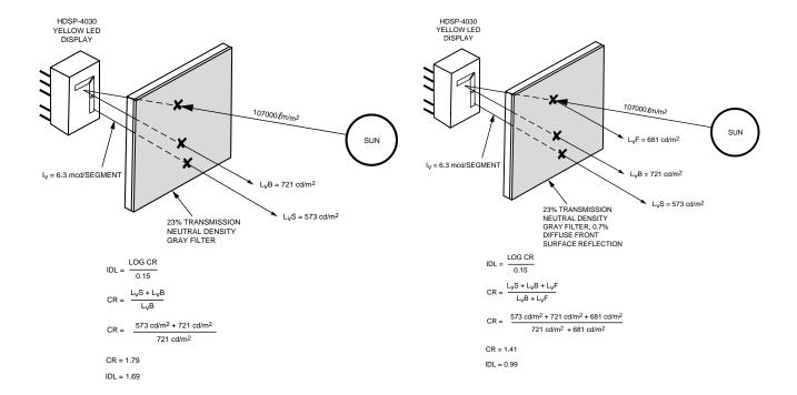
Figure 24. Luminance Index — No Front Surface Reflectance.
