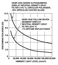
Figure 47. Effect of Reducing Ambient Lighting.
