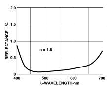
Figure 36. Front Surface Reflectance of Glass with Double Sided 1/4 Wave Optical Coating.
