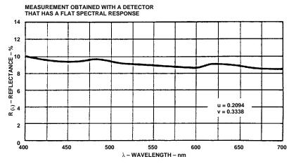
Figure 23. Reflectance Characteristic for the Face of a Gray Body Stretched Segment Sunlight Viewable LED Display.
