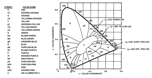
Figure 19. Dominant Wavelengths and Corresponding Colors for LEDs, Shown on the CIE Chromaticity Diagram.
