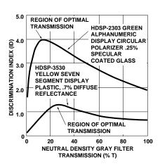
Figure 46. Optimal Neutral Density Gray Filter Transmission.
