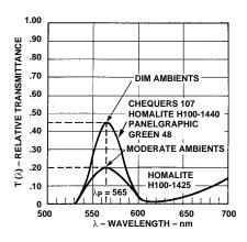
Figure 9. Typical Transmittance Curves for Filters to be used with Green Displays.
