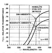
Figure 7. Typical Transmittance Curves for Filters to be used with High Efficiency Red Displays.
