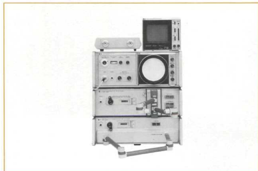
Figure 2-16. HP 8410S Option 310 0.11 – 12.4 GHz
