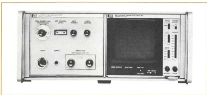
Figure 2-5. The Phase-Magnitude Display Plug-In
