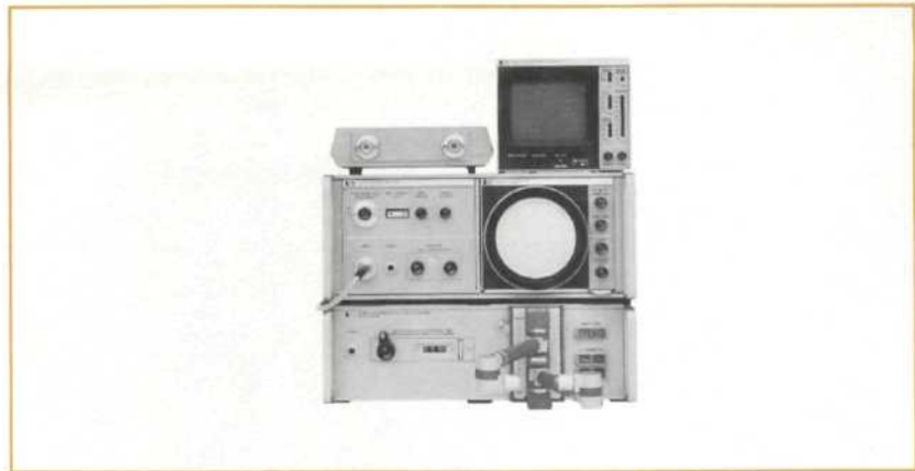
Figure 2-14. HP 8410S Option 110 0.11 – 2 GHz
