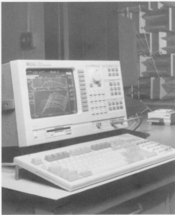
Figure 3: The HP 35665A is a two-channel real-time analyzer that can be programmed to control a multiplexer for automated measurements.
