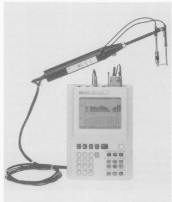
Figure 4: Newer 1/3-octave real-time analyzers with intensity probes can measure both pressure and particle velocity at the same time.
