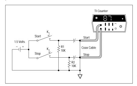
Figure 39. Simple Time Interval measuring System
