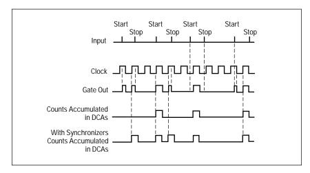
Figure 23. Synchronizer operation with time interval averaging.
