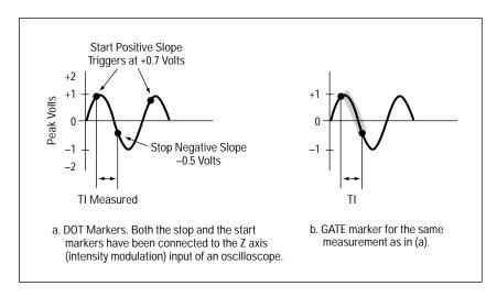
Figure 18. Time Interval Markers as they appear on an oscilloscope.
