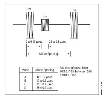
Figure 41. Three-pulse ATC ground station interrogation.
