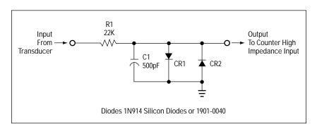
Figure 8. Simple clipper circuit to prevent counter input overload.
