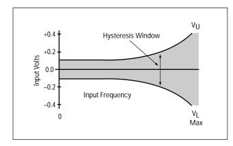
Figure 17. Hysteresis window gets wider if input sensitivity decreases with increasing frequency.
