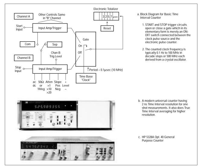
Figure 2. Measuring Time Interval with an Electronic Counter
