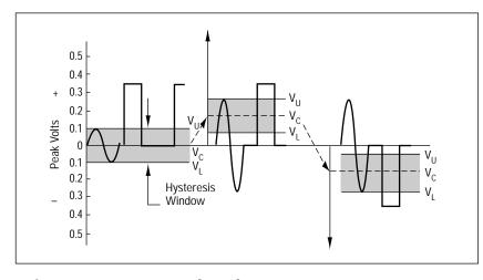
Figure 11. Polarity and Level Controls
