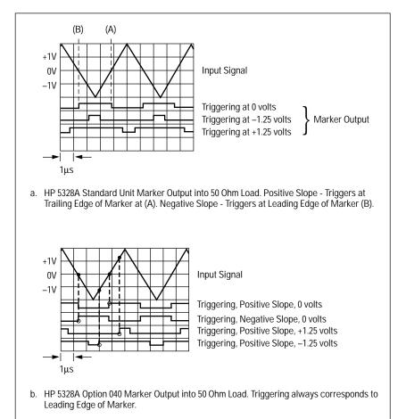
Figure 21. Square wave marker output of the HP 5328A Counter.
