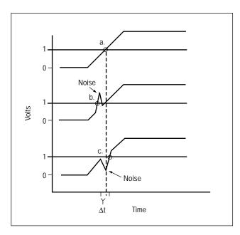
Figure 25. Time Error introduced by noise on the input signal.
