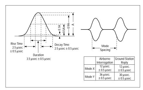
Figure 45. DME Pulse characteristic
