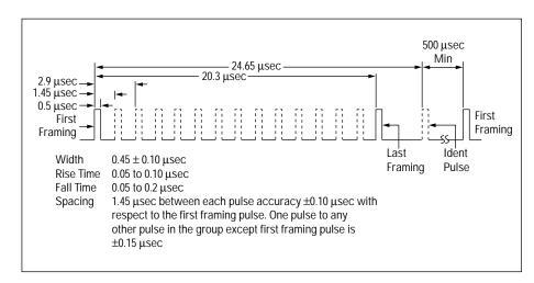
Figure 42. Available ATC reply Pulse codes.
