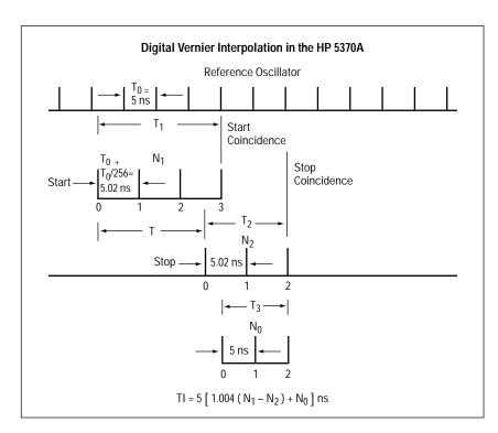
Figure 32. Digital Interpolation Scheme using phase-startable phase-lockable oscillators.
