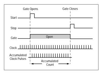
Figure 1. In a time interval measurement, clock pulses are accumulated for the duration the main gate is open. The gate is opened by one event, START and closed by the other, STOP.
