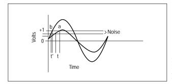
Figure 27. Increased signal amplitude reduces time error.
