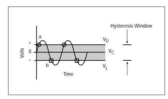
Figure 15. Triggering on positive or negative slope.
