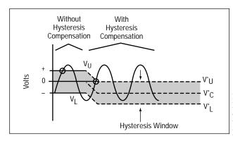
Figure 16. Hysteresis compensation for triggering on a positive slope.
