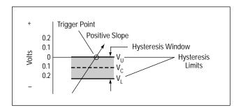
Figure 12. To trigger at a particular voltage (zero volts dc in this example) with a positive slope. Upper and lower hysteresis limits are positioned as shown above.
