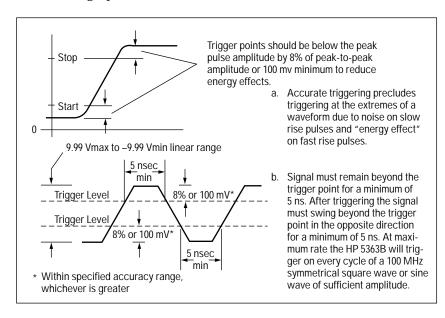
Figure 38. Input Signal requirements for the HP 5363B.
