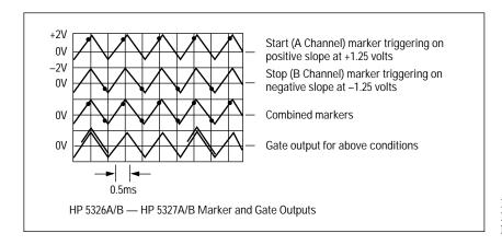
Figure 19. Actual Dot and Gate Marker Outputs
