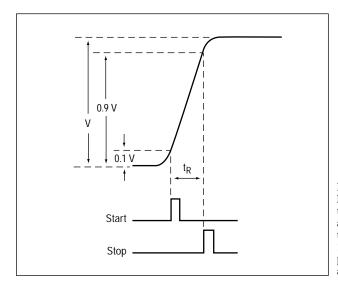
Figure 3. Measuring the rise time t<sub>R</sub> by adjusting the trigger levels to the 10% and 90% points of the input amplitude.
