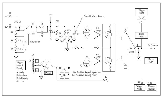
Figure 6. Symmetrical Input Amplifier Trigger Circuit for Time Interval Counter.
