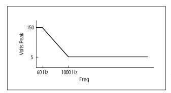
Figure 7. Overload voltage as a function of frequency.
