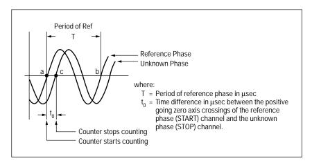
Figure 40. Phase measurement with a time interval counter.
