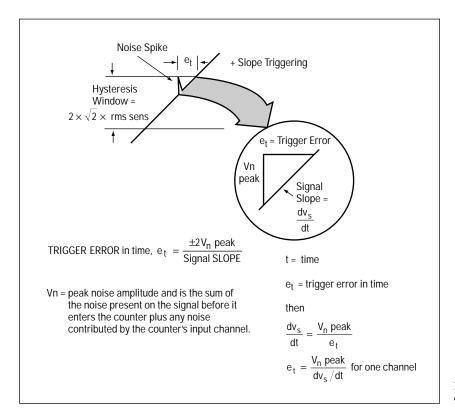
Figure 30. Trigger error derivation
