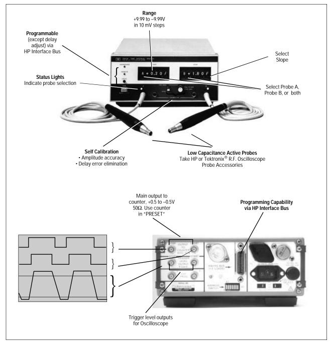
Figure 37. HP 5363B Controls and Connectors
