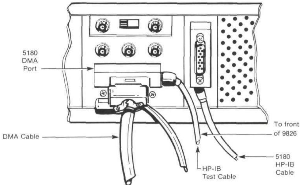
Figure 4. Cable configuration to allow DMA interface control line logic levels to be monitored during DMA transfer.
