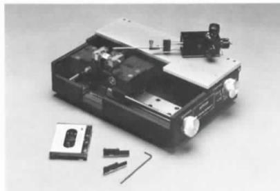
Figure 27. Coaxial to microstrip adaptor
