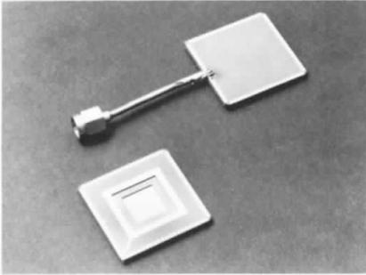
Figure 29. Short semirigid on IC package pad
