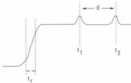
If  $t_2 - t_1 \leq 0.5 \times t_r$ , then two reflections merge as one pulse.
