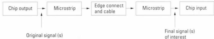
**Figure 11. Typical digital circuit transmission path**
