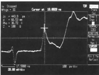
Figure 30. TDR Response to IC package path
