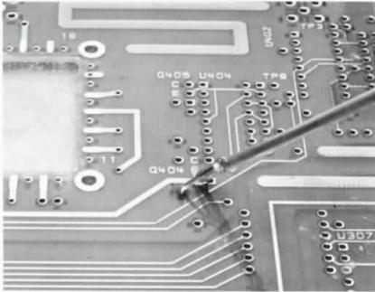
Figure 16. Semirigid onto trace with via holes
