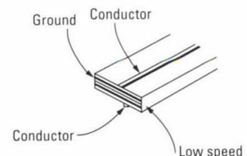
Figure 14. Controlled impedance lines
