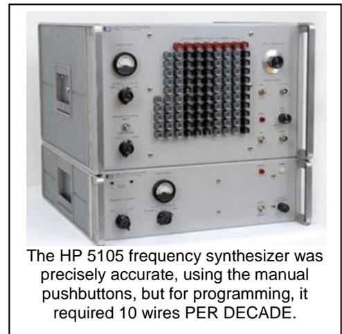
Then we came to the HP 5100 frequency synthesizer family from Bagley's F&T Division. Customers needed this capability for programmable stimulus signals for their test systems. The synthesizer had ten push buttons on each decade, so there were ten wires for each decade of the frequency input. We at AMD had pretty much standardized on BCD code, so one of our first custom designs was a decoder from BCD to ten wires to run the synthesizer. This was needed for all 10 digits of input of the 5100.
