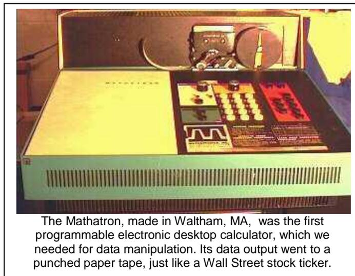
The Mathatron, made in Waltham, MA, was the first programmable electronic desktop calculator, which we needed for data manipulation. Its data output went to a punched paper tape, just like a Wall Street stock ticker.
