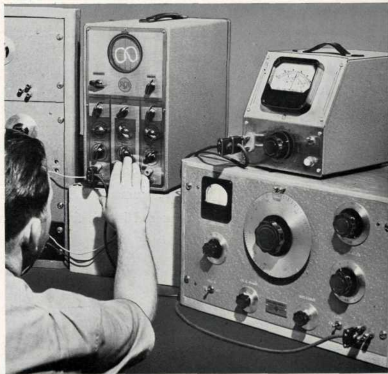
A Model 205A being checked on the frequency standard in the -hp- laboratory. Notice the Model 400A Vacuum Tube Voltmeter.
