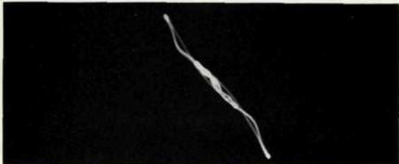
Square wave applied to two amplifiers, output of one on horizontal plates, output of other vertical plates for rapid comparison test. Nearly straight line obtained when amplifiers have nearly identical characteristics.
