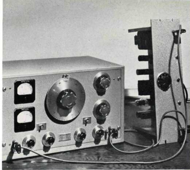
A Model 205AG is connected to measure the gain of an amplifier.
