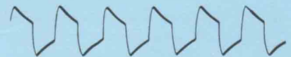
2. Square wave distortion from poor response at both high and low frequencies.
