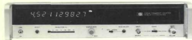
5341A (option 011) Automatic Frequency Counter. 10 Hz to 4.5 GHz, fast measurements
