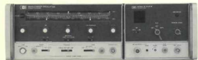
8620A (option E45) Microwave Sweep Oscillator. 3 MHz to 18 GHz (2-18 GHz with one plug-in)
