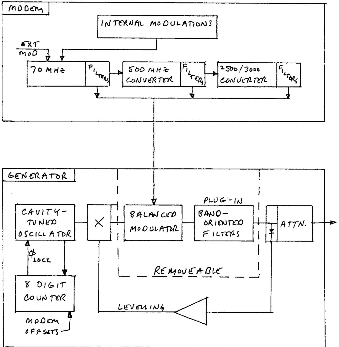
The cavity is phase-lock stabilized and counted for 1 kHz or 10 kHz resolution. Automatic sensing from the modem offsets the counter so that the actual output frequency is displayed. The cavity output could also be used directly and would yield  $\approx 10\text{MW}$ . When mixed and used with the modem, signal output would be approximately -10 dBm to -120 dBm.
