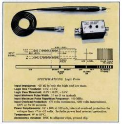
Figure A1, 10525T Logic Probe.
