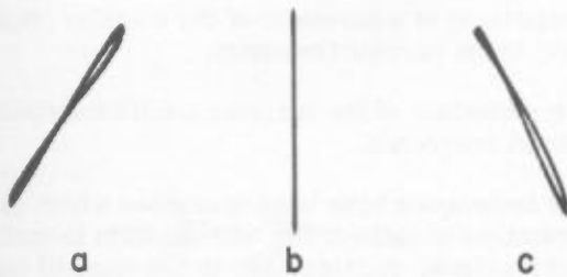
Fig. 10. Pointer Presentation for CW signal (a) below, (b) "on", and (c) above harmonic of Transfer Oscillator
