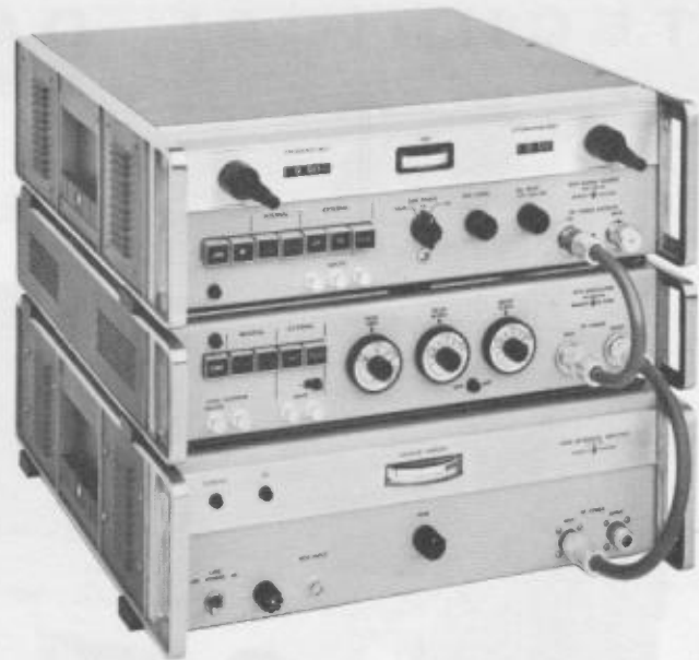
Figure 1. \Phi Models 8614A, 8714A, and 489A form a sophisticated 1-watt source for frequencies from 1 to 2 gc.
