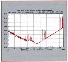
The HP 3048A was designed to plot the measured noise data in any of several output formats;  $\mathcal{L}(f)$ ,  $S_{\phi}(f)$ ,  $S_{\psi}(f)$  or  $S_{\psi}(f)$ .
