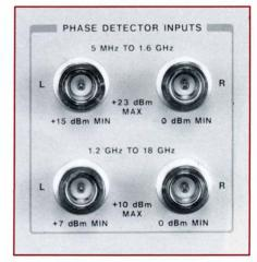
The HP 3048A's standard frequency range of 5 MHz to 1.6 GHz covers RF sources and devices that need phase noise characterization.
