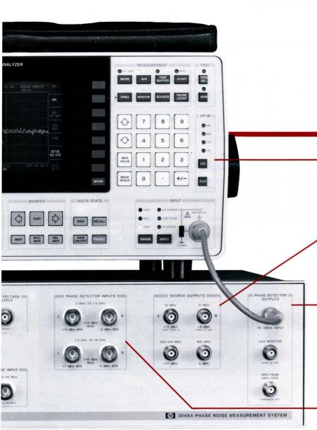
The HP 3561A measures the noise data to a maximum of 100 kHz offset frequency. It is also extensively used for system calibration and real-time noise monitoring.
