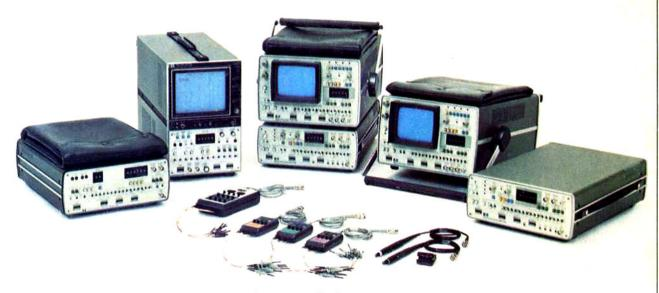
Your choice in data domain instrumentation is growing steadily. It extends from simple 4-bit AND gate trigger probes, to an optional Logic State Switch on HP scopes for selecting either time or data domain, to the 1600S—the system with up to 32 channels plus qualifier inputs, storage, delay, and two modes of display (table or map). There's an instrument or accessory in this family to put you in the data domain and give you a much better view of your digital designs.
